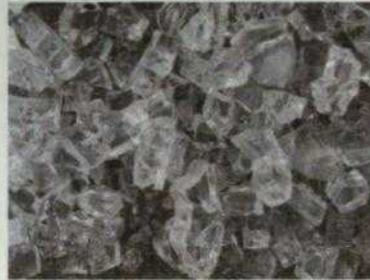
Broken glass is used by factories to lower the temperature of their furnaces. It is also separated by colour and blown into cheap bottles in Mahalaxmi and Kurla. Broken glass from Bombay is
